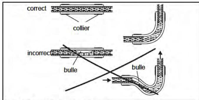
Fig. 14: Raccordement tube-tuyau
